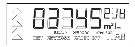
MULTICAL® 21 can be read from the big, easily readable, specially designed display. The five big figures indicate number of cubic metres. The three small figures are decimals.
